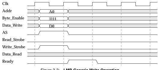
Figure 2-2: LMB Generic Write Operation
